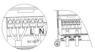
**Note:** The grounding wire shall be as thick as possible (cross-sectional area is not less than 4mm2). The grounding point shall be as close as possible to the all-in-one solar charge inverter. The shorter the grounding wire, the better.
